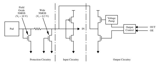
Figure 1. 3-V/5-V Input Compatible I/O Structure
