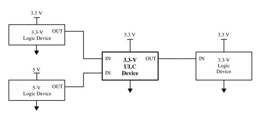
Figure 2. Simple Example of Mixed Power Supply Circuitry
