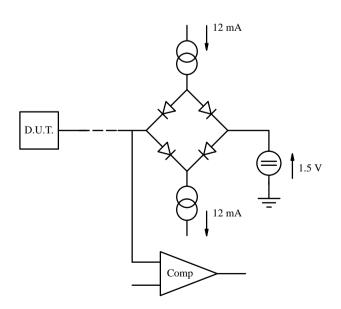
Figure 3. Typical ULC Test Conditions
