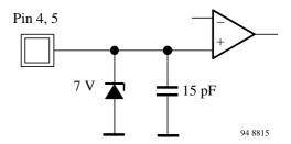
Figure 3b Input circuit Pin 4 and Pin 5
