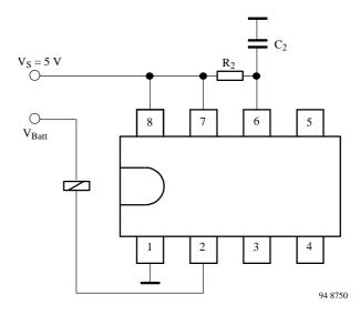
Figure 2b Basic circuit for  $V_S = 5 \text{ V}$
