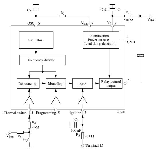
Figure 1 Block diagram with external circuit
