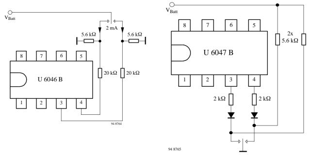
Figure 10 Increasing the contact current by parallel resistors
