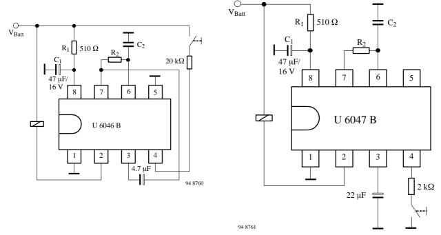
Figure 8 Generation of a monostable delay time,  $t_{d,}$  by applying the operating voltage  $V_{Batt,}$  deactivatable by the OFF push-button
