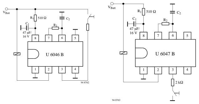
Figure 9 Monostable delay time,  $t_d$ , can be activated by the ON push-button, not externally deactivatable
