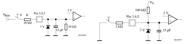
Figure 6a Input circuit U 6046 B
