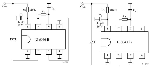
Figure 7 Generation of a monostable delay time,  $t_d$ , caused by applying the operating voltage  $V_{Batt}$ , not externally deactivatable.
