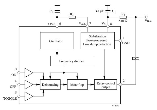
Figure 1 Block diagram with external circuit
