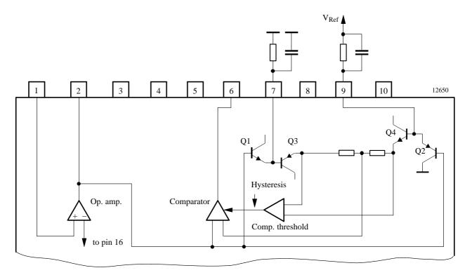
Figure 3. Principle function of the clamping comparator
