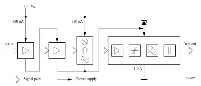
Figure 29. Principle diagram UHF remote control receiver
