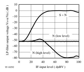
Figure 24. Signal to noise ratio AM
