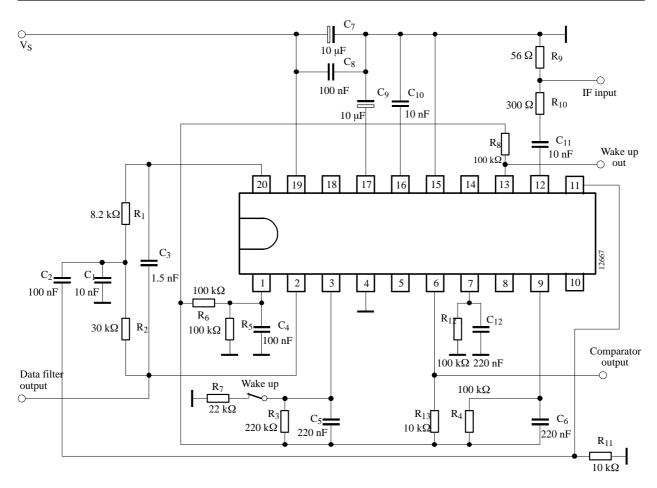
Figure 23. AM test circuit with 2 kHz Bessel low pass data filter
