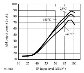
Figure 25. AM-demodulator characteristic vs. temperature
