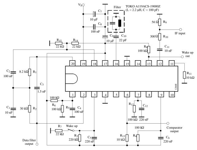
Figure 26. FM test circuit with 2 kHz Bessel low pass data filter
