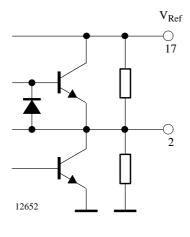
Figure 5. Pin 2 OP<sub>out</sub>
