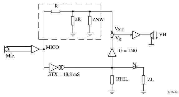
Figure 7. Schematic of the side tone
