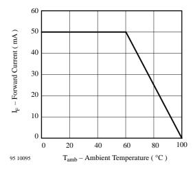
Figure 2. Forward Current vs. Ambient Temperature
