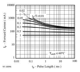
Figure 3. Forward Current vs. Pulse Length
