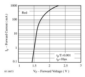
Figure 5. Forward Current vs. Forward Voltage
