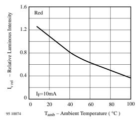
Figure 6. Rel. Luminous Intensity vs. Ambient Temperature
