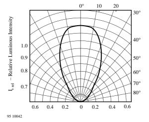
Figure 4. Rel. Luminous Intensity vs. Angular Displacement
