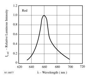
Figure 9. Relative Luminous Intensity vs. Wavelength
