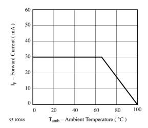
Figure 2. Forward Current vs. Ambient Temperature
