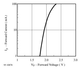
Figure 4. Forward Current vs. Forward Voltage
