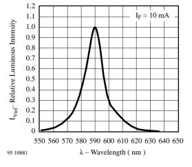
Figure 8. Relative Luminous Intensity vs. Wavelength
