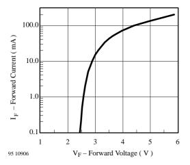
Figure 4. Forward Current vs. Forward Voltage
