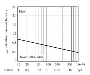
Figure 6. Rel. Lumin. Intensity vs. Forw. Current/Duty Cycle
