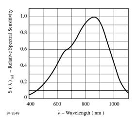
Figure 8. Relative Spectral Sensitivity vs. Wavelength
