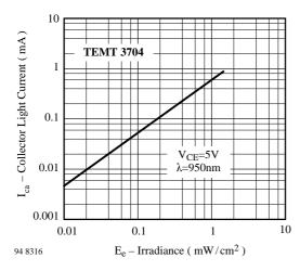
Figure 4. Collector Light Current vs. Irradiance
