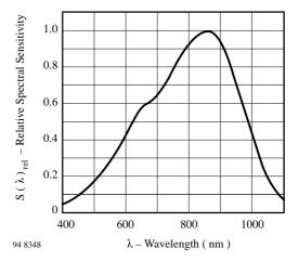
Figure 8. Relative Spectral Sensitivity vs. Wavelength
