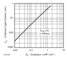
Figure 4. Collector Light Current vs. Irradiance
