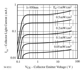
Figure 5. Collector Light Current vs. Collector Emitter Voltage
