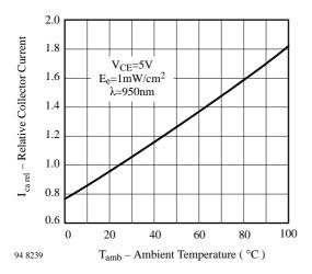
Figure 3. Relative Collector Current vs. Ambient Temperature
