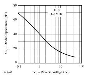
Figure 5. Diode Capacitance vs. Reverse Voltage
