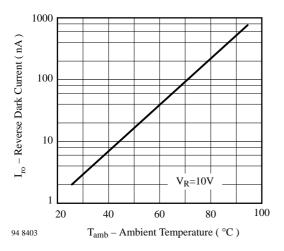
Figure 1. Reverse Dark Current vs. Ambient Temperature
