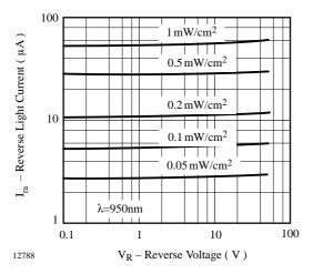
Figure 4. Reverse Light Current vs. Reverse Voltage
