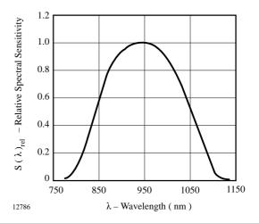
Figure 6. Relative Spectral Sensitivity vs. Wavelength
