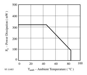
Figure 1. Power Dissipation vs. Ambient Temperature
