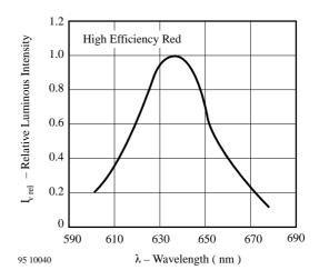
Figure 8. Relative Luminous Intensity vs. Wavelength
