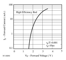
Figure 4. Forward Current vs. Forward Voltage
