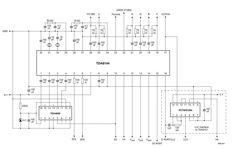
Pins 28 and 32 are sensitive to leakage currents.
