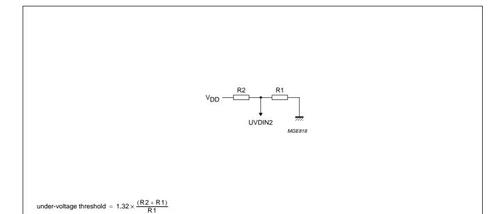
Fig.8 Reset mode threshold.
