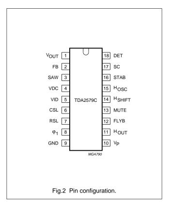
divider system for generating the vertical sawtooth at pin 3. Thus no vertical frequency adjustment is required.
