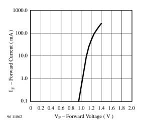
Figure 4. Forward Current vs. Forward Voltage
