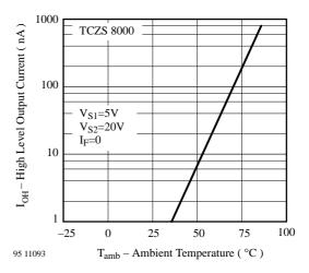
Figure 7. High Level Output Current vs. Ambient Temp.
