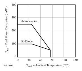
Figure 3. Total Power Dissipation vs. Ambient Temperature
