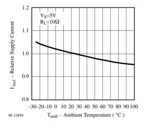
Figure 5. Relative Supply Current vs. Ambient Temperature
