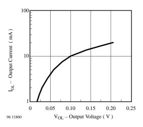
Figure 6. Output Current vs. Output Voltage
