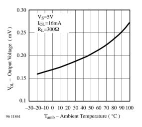
Figure 7. Output Voltage vs. Ambient Temperature
