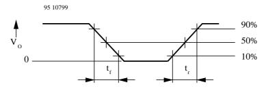
Figure 2. Pulse diagram
