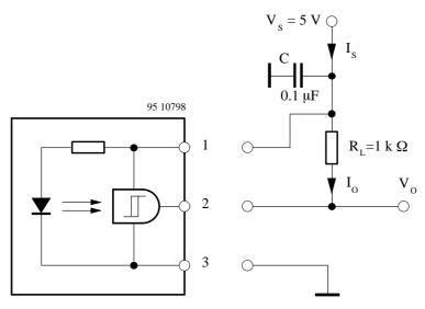
Figure 1. Test circuit and pin connection
