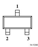
Marking: 852 Plastic case (SOT 23) 1 = Collector; 2 = Base; 3 = Emitter
