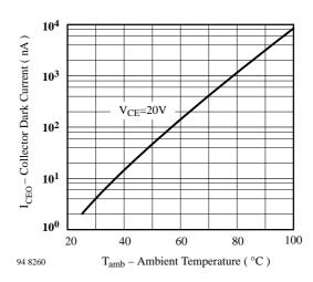
Figure 2. Collector Dark Current vs. Ambient Temperature
