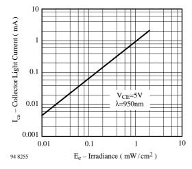
Figure 4. Collector Light Current vs. Irradiance
