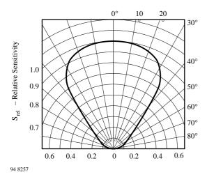
Figure 9. Relative Radiant Sensitivity vs. Angular Displacement
