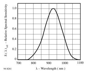
Figure 8. Relative Spectral Sensitivity vs. Wavelength
