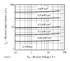
Figure 5. Reverse Light Current vs. Reverse Voltage
