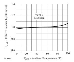
Figure 2. Relative Reverse Light Current vs. Ambient Temperature
