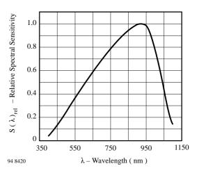
Figure 7. Relative Spectral Sensitivity vs. Wavelength
