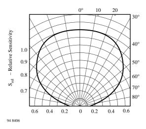
Figure 8. Relative Radiant Sensitivity vs. Angular Displacement
