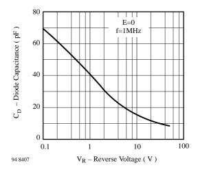
Figure 6. Diode Capacitance vs. Reverse Voltage
