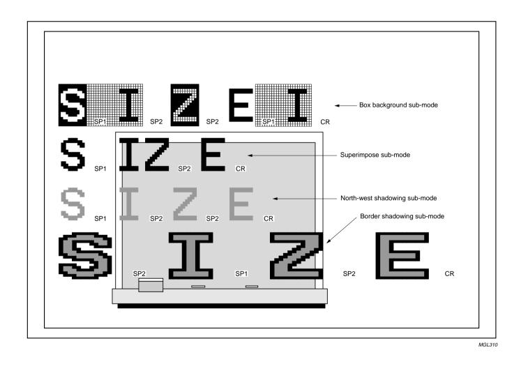
Fig.37 SP1 and SP2 codes in the 4 sub-modes of TV mode.
