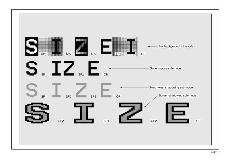
Fig.38 SP1 and SP2 codes in the 4 sub-modes of Frame mode.
