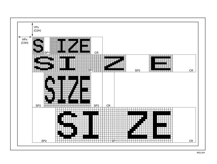
Fig.29 An example of flexible display format (Split space on).
