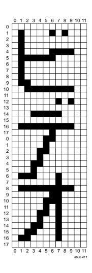
Fig.42 Combination of two font cells in a vertical direction.
