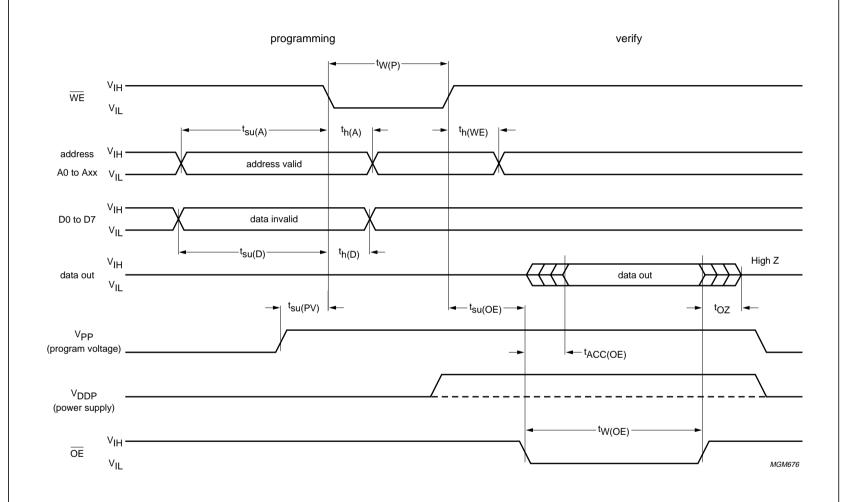
V<sub>IH</sub> and V<sub>IL</sub> are CMOS levels and are typically 5 V and 0 V respectively.
