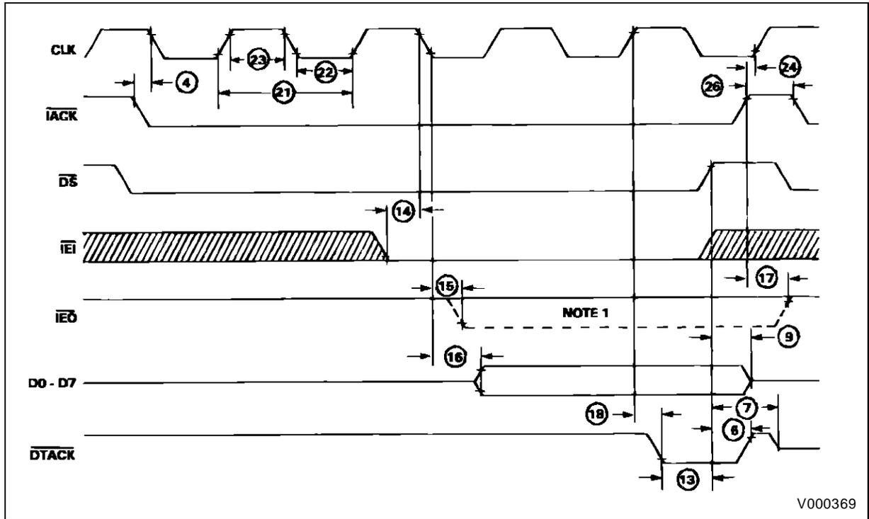
Figure 24 : Interrupt Acknowledge Cycle ( $\overline{IEI}$  high).
