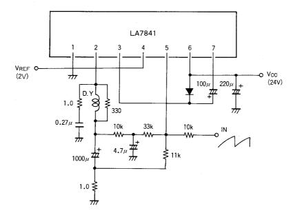
Unit (resistance:  $\Omega$ , capacitance: F)
