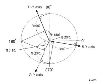
8. Calculate the AF angle with the following formula, where BR is the B-Y/R-Y demodulation output ratio and  $\theta$  is ANGBR, the B-Y/R-Y demodulation angle.
