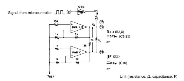
The design of the above when mute is ON (pin 16 open) is as follows:
