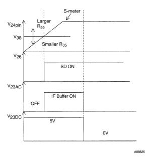
Pin 55: AM SD Adjustment Pin
