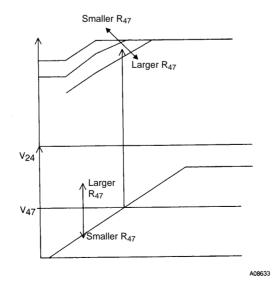
By comparing the pin 47 mute on adjustment voltage to the S-meter voltage (V24), the muting on point can be adjusted.
