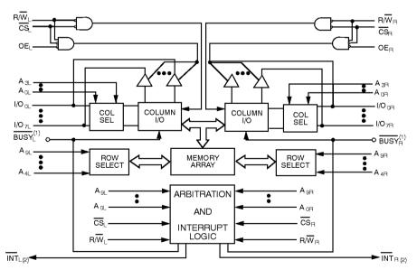
Notes: 1. L 67130 (MASTER): BUSY is open drain output and requires pullup resistor
