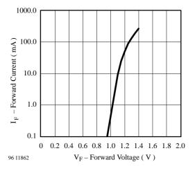
Figure 4. Forward Current vs. Forward Voltage
