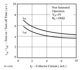
Figure 12. Turn on / off Time vs. Collector Current
