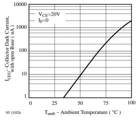
Figure 6. Collector Dark Current vs. Ambient Temperature
