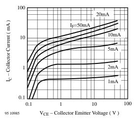
Figure 8. Collector Current vs. Collector Emitter Voltage
