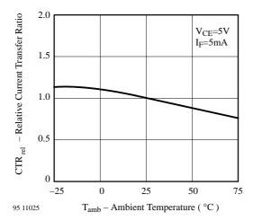
Figure 5. Rel. Current Transfer Ratio vs. Ambient Temperature
