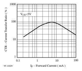
Figure 10. Current Transfer Ratio vs. Forward Current
