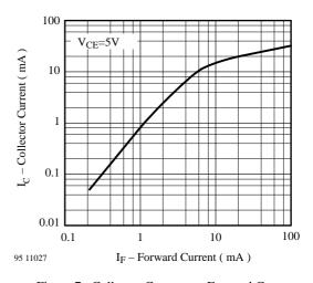
Figure 7. Collector Current vs. Forward Current
