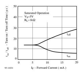
Figure 11. Turn on / off Time vs. Forward Current
