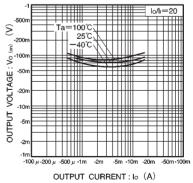
Fig.4 Output voltage vs. output current
