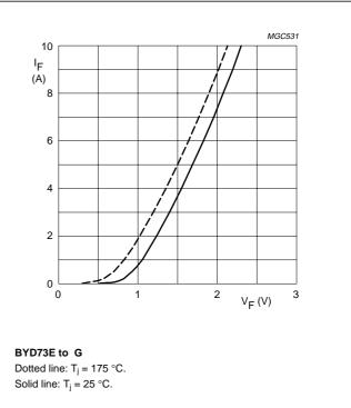
Fig.13 Forward current as a function of forward voltage; maximum values.
