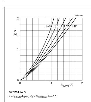
Fig.10 Maximum steady state power dissipation (forward plus leakage current losses, excluding switching losses) as a function of average forward current.
