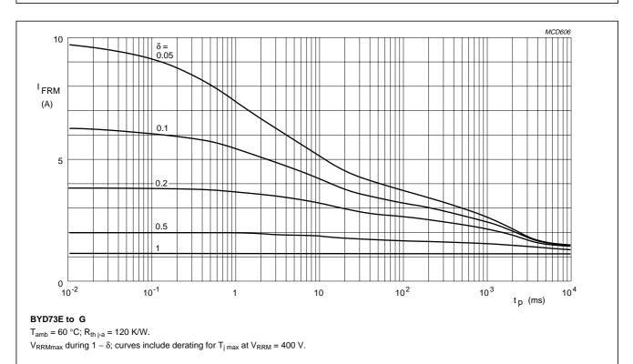
Fig.9 Maximum repetitive peak forward current as a function of pulse time (square pulse) and duty factor.
