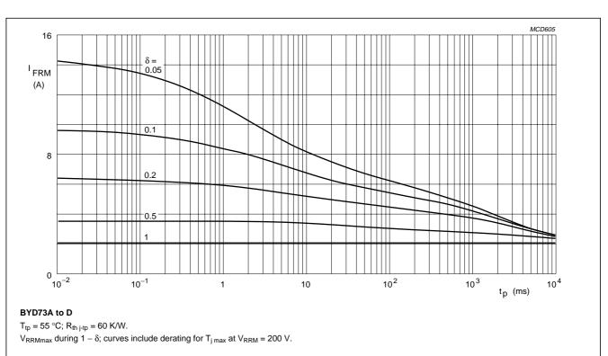
Fig.6 Maximum repetitive peak forward current as a function of pulse time (square pulse) and duty factor.
