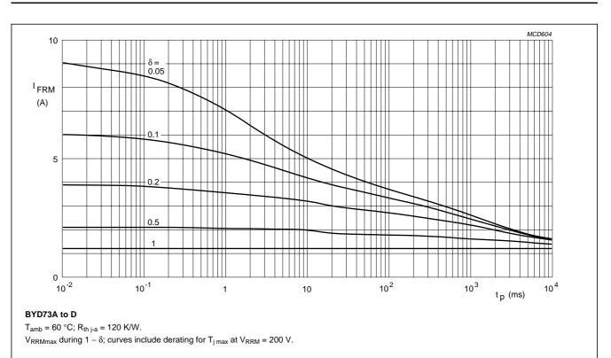
Fig.8 Maximum repetitive peak forward current as a function of pulse time (square pulse) and duty factor.
