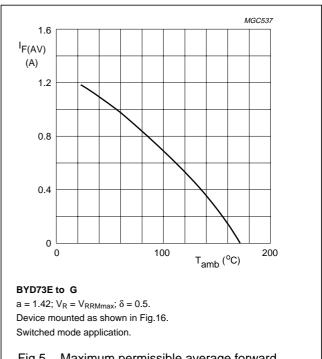
Fig.5 Maximum permissible average forward current as a function of ambient temperature (including losses due to reverse leakage).
