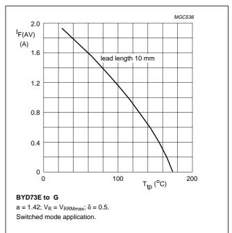
Fig.3 Maximum permissible average forward current as a function of tie-point temperature (including losses due to reverse leakage).
