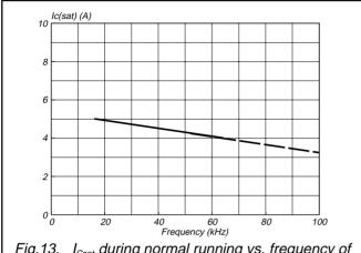
Fig.13. I<sub>Csat</sub> during normal running vs. frequency of operation for optimum performance
