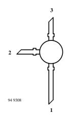
BF970 Marking: BF970 Plastic case (TO 50) 1= Collector; 2= Base; 3= Emitter
