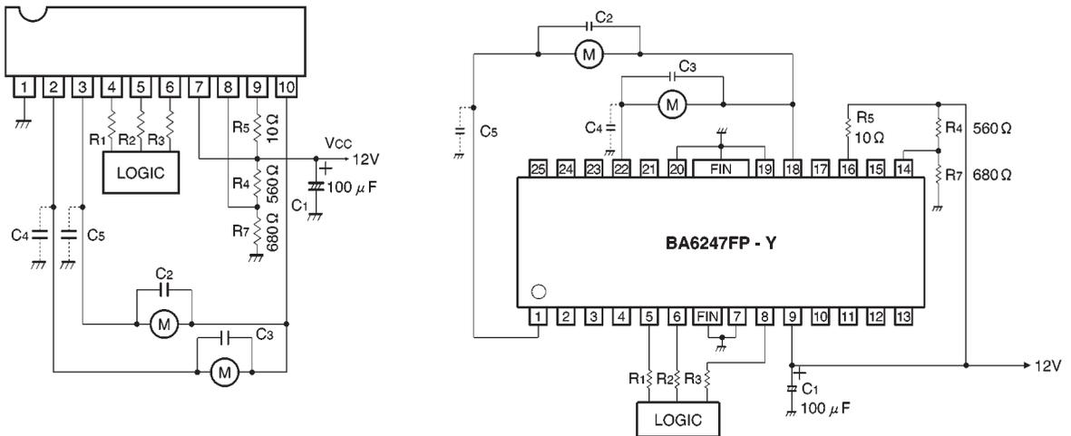
C2, C3: Capacitors for preventing parasitic oscillation. Though the optimum capacitance depends on such PCB arrangement factors as the power supply circuit, motor characteristics, and conductor foil patterns, a range of 0.011  $\mu\text{F}$  is recommended.
