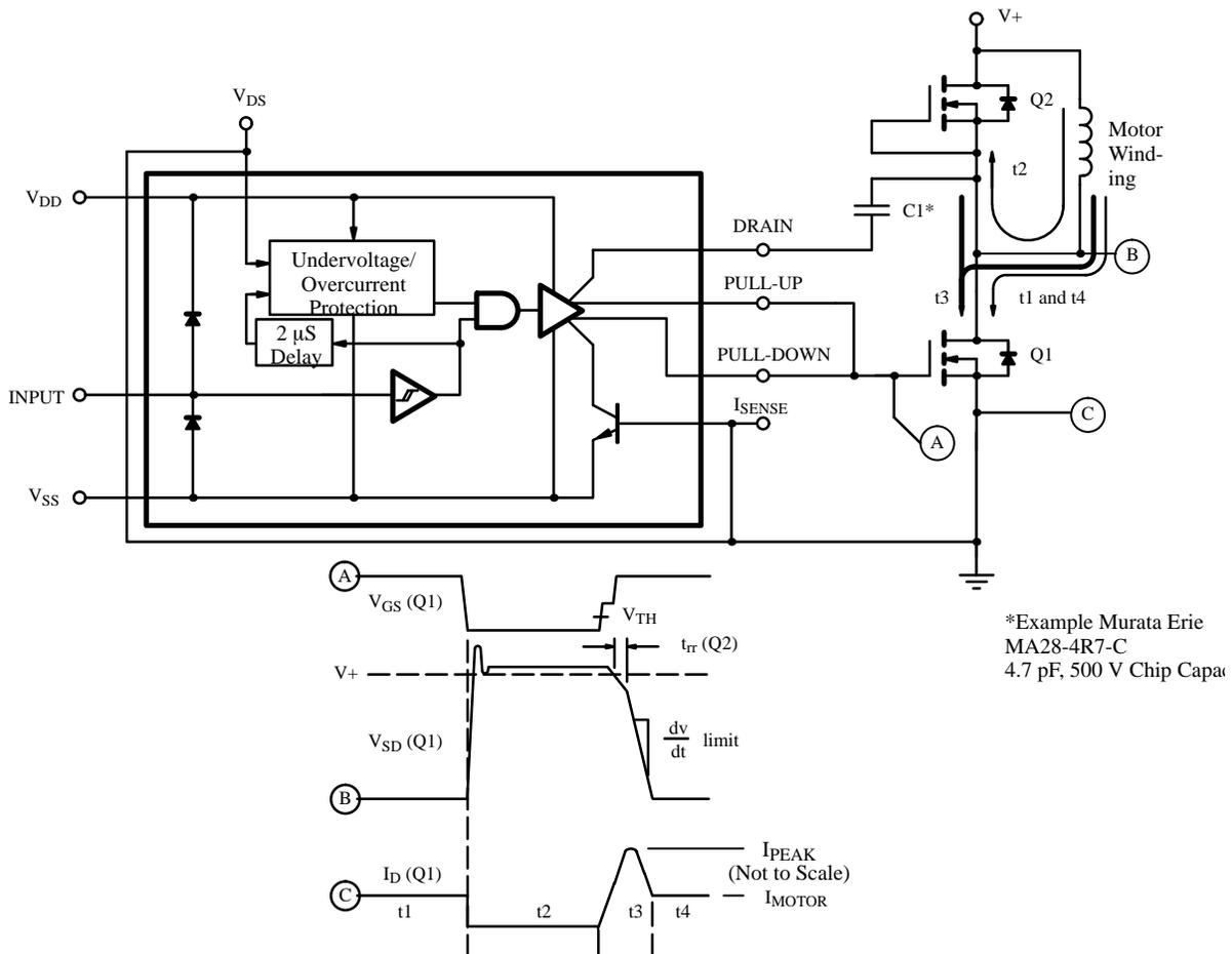
Figure 7. Direct  $dv/dt$  Limiting
