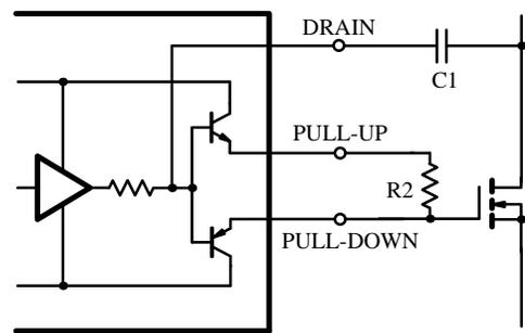
Figure 6. Simplified dv/dt Feedback Circuit
