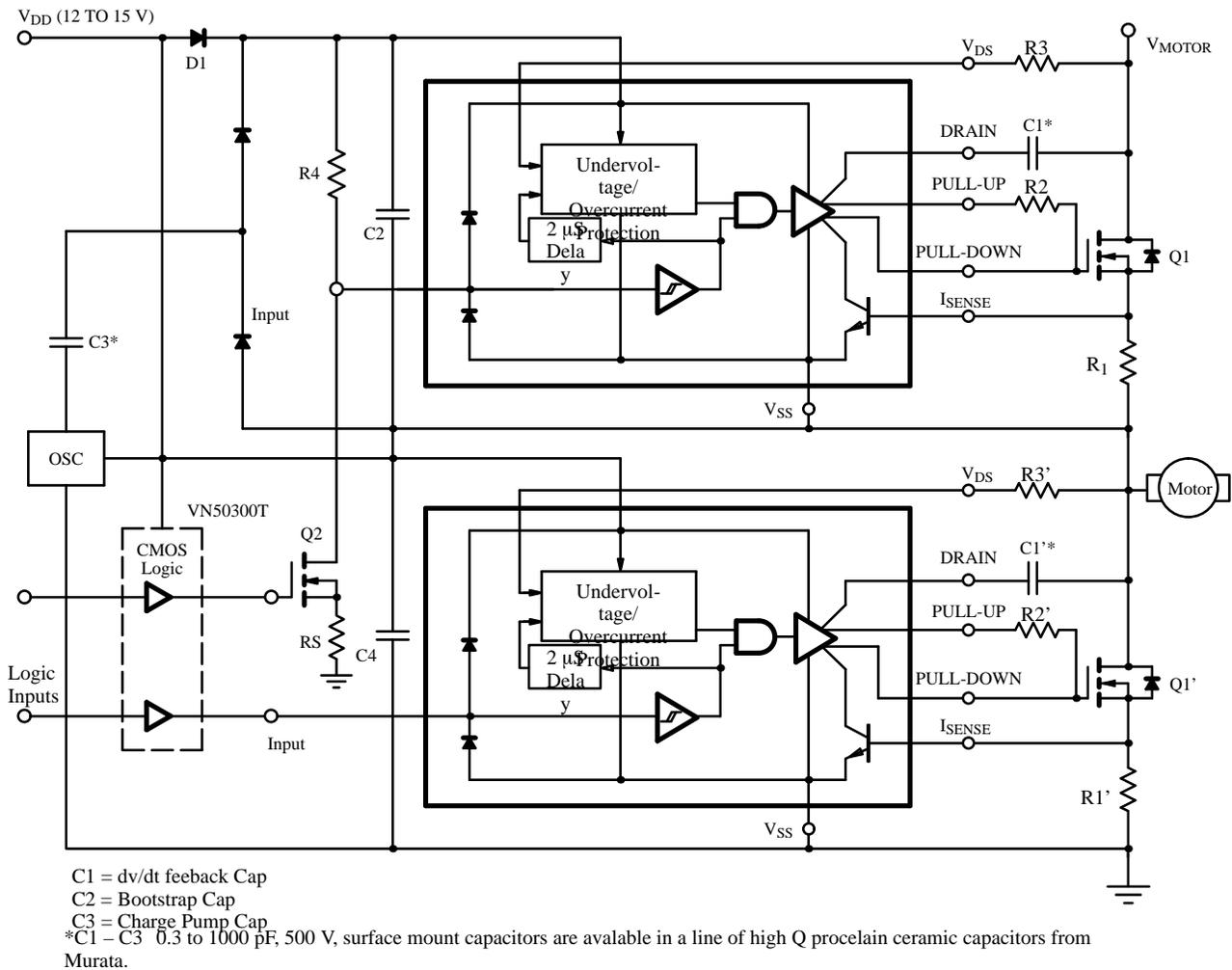
**Figure 8.** High-Voltage Half-Bridge with Si9910 Drivers
