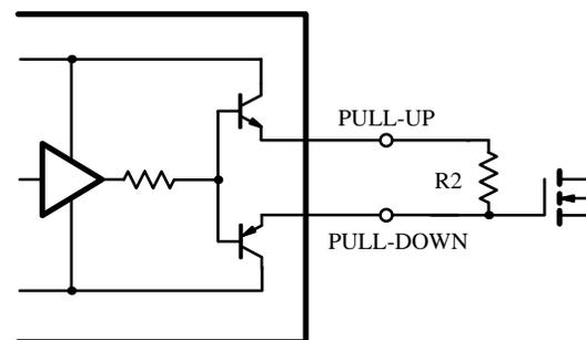
Figure 3a. Simplified "Split" Emitter-Follower Output Circuit
