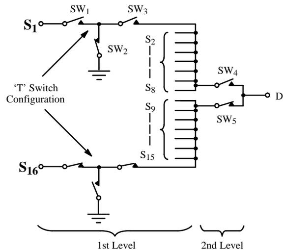
Figure 2. Switch Configuration
