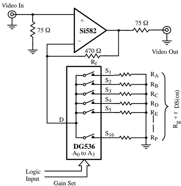
**Figure 18.** Programmable Gain Video Amplifier
