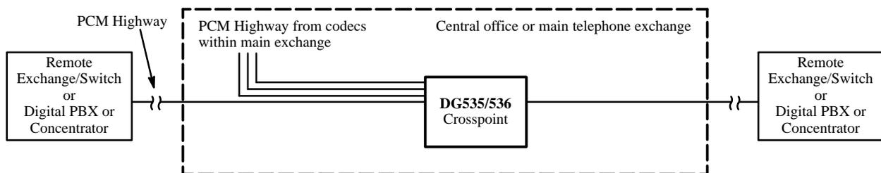
**Figure 17.** DG536 PCM Distribution Frame
