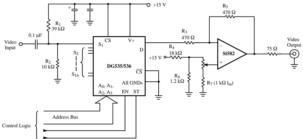
**Figure 7.** General-Purpose 16-Channel Wideband Multiplexer
