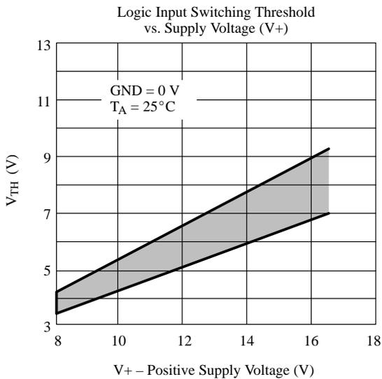
**Figure 9.** Logic Input Switching Threshold vs. Supply Voltage
