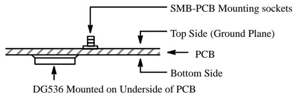
**Figure 6.** Circuit Board Layout for Optimal Performance (DG536)
