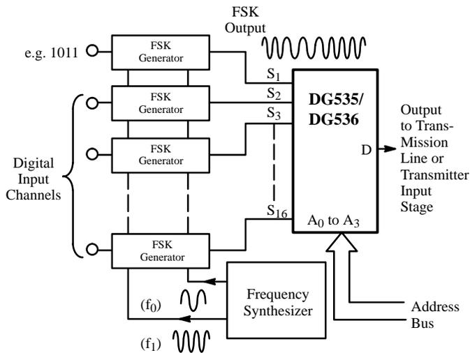
**Figure 14.** FSK Multiplexing System Block Diagram
