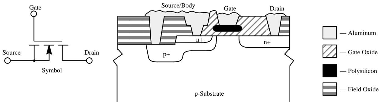
**Figure 3.** Cross-Section of an N-Channel, Silicon-Gate DMOS Transistor
