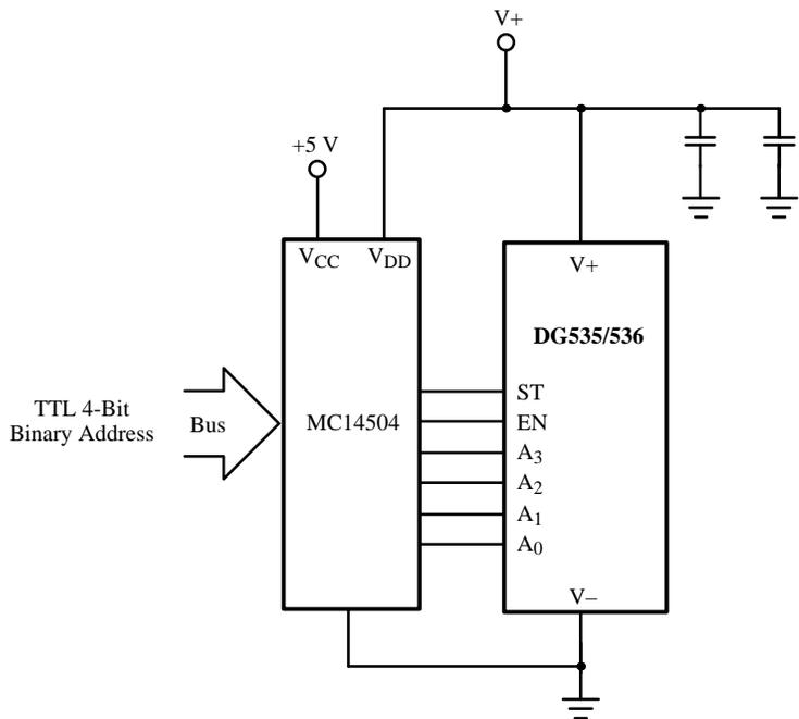
**Figure 10.** Using the MC14504 for Address Logic Level Shifting
