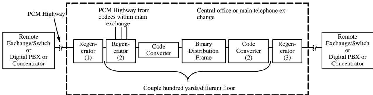
**Figure 16.** Binary PCM Routing Network
