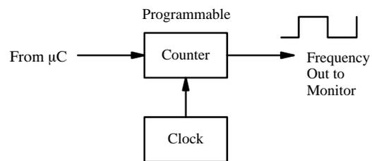
**Figure 5.** Pulse Rate Simulator
