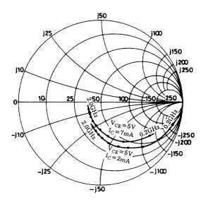
$V_{CE} = 5V$ f = 200 to 2000MHz (200MHz Step)
