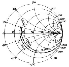
$\begin{array}{l} S21e:V_{CE}\!=\!5V\\ f\!=\!100,200\,{\rm to}\,2000MHz\,(200\ step\,) \end{array}$
