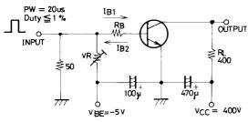
Unit (resistance: Ω, capacitance: F)
