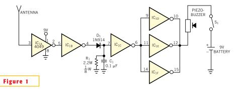
A low level at the outputs of  $\rm IC_{1D}$  ,  $\rm IC_{1E}$  , and  $\rm IC_{1F}$  activates the piezo-buzzer and warns of ac-line failure.
