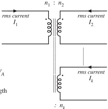
Q: how should the window area  $W_A$  be allocated among the windings?
