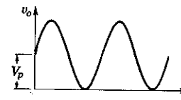
FIGURE 4-38 Negative peak of output waveform is clamped at zero when V = 0 in diode clamp circuit of Fig. 4-37.
