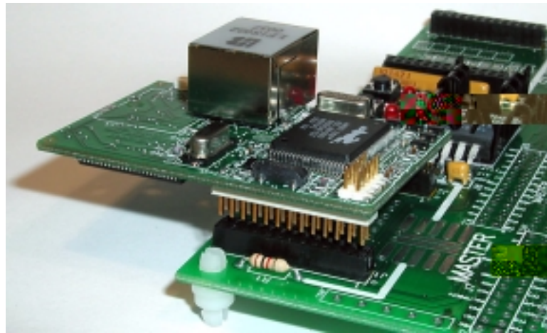
Figure 2–3: Installing the RCM2200 module on the Prototyping Board.
