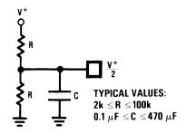
(a) Resistive Divider with Decoupling Capacitor
