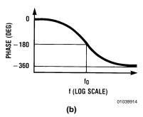
$$H_{AP}(s) = \frac{H_{OAP}\left(s^2 - \frac{s\omega_{O}}{Q} + \omega_{O}^2\right)}{s^2 + \frac{s\omega_{O}}{Q} + \omega_{O}^2}$$
