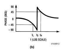
$$\begin{split} &H_{\text{N}}(s) = \frac{H_{\text{ON}}(s^2 + \omega_{\text{O}}^2)}{s^2 + \frac{s\omega_{\text{O}}}{Q} + \omega_{\text{O}}^2} \\ &Q = \frac{f_{\text{O}}}{f_{\text{H}} - f_{\text{L}}}; \; f_{\text{O}} = \sqrt{f_{\text{L}} \, f_{\text{H}}} \\ &f_{\text{L}} = f_{\text{O}} \left( \frac{-1}{2Q} + \sqrt{\left( \frac{1}{2Q} \right)^2 + 1} \; \right) \\ &f_{\text{H}} = f_{\text{O}} \left( \frac{1}{2Q} + \sqrt{\left( \frac{1}{2Q} \right)^2 + 1} \; \right) \end{split}$$
