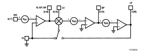
FIGURE 19. MF10 Offset Voltage Sources
