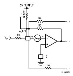
FIGURE 20. Method for Trimming  $V_{\text{OS}}$
