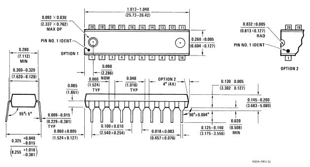
20-Lead Molded Dual-In-Line Package (N) Order Number MF10ACN or MF10CCN **NS Package Number N20A**
