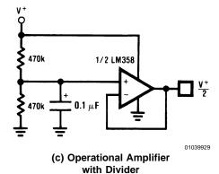
FIGURE 18. Three Ways of Generating V\*/2 for Single-Supply Operation
