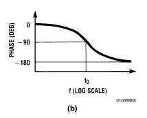
$$\begin{split} & \textbf{H}_{LP}(\textbf{s}) = \frac{\textbf{H}_{OLP}\omega_{O}^{2}}{\textbf{s}^{2} + \frac{\textbf{s}\omega_{O}}{Q} + \omega_{O}^{2}} \\ & \textbf{f}_{C} = \textbf{f}_{O} \times \sqrt{\left(1 - \frac{1}{2Q^{2}}\right) + \sqrt{\left(1 - \frac{1}{2Q^{2}}\right)^{2} + 1}} \\ & \textbf{f}_{p} = \textbf{f}_{O} \sqrt{1 - \frac{1}{2Q^{2}}} \\ & \textbf{H}_{OP} = \textbf{H}_{OLP} \times \frac{1}{\frac{1}{Q}\sqrt{1 - \frac{1}{4Q^{2}}}} \end{split}$$
