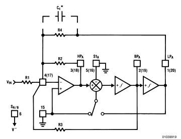
\*In Mode 3, the feedback loop is closed around the input summing amplifier; the finite GBW product of this op amp causes a slight Q enhancement. If this is a problem, connect a small capacitor (10 pF – 100 pF) across R4 to provide some phase lead.
