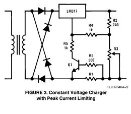
Idjustable 3-Terminal Regulator for Low-Cost Battery Charging Systems
