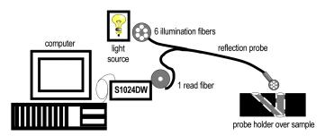
A typical configuration for a reflection experiment.
