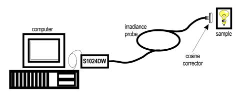
A typical configuration for an irradiance experiment.
