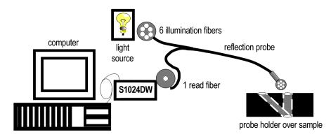
A typical configuration for a reflection experiment.
