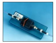
FHS In-Line Filter Holders for the UV-VIS-NIR or VIS-NIR provide a convenient platform for rapid absorbance or transmission measurements of optical and other filters. Filter holders come with a pair of 5-mm diameter collimating lenses, and accept 1" round or any size square optical filters, up to 6 mm in thickness. FHS assemblies are typically used either to measure filters or to put filters into optical setups.
