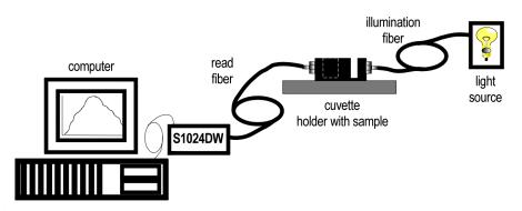
A typical configuration for an absorbance experiment.
