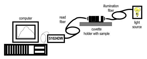
A typical configuration for a transmission experiment.
