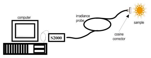
A typical configuration for an irradiance experiment.
