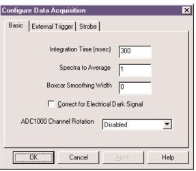
amount of light you anticipate for your application causes a signal of ~3500 counts while in scope mode. The *actual* integration time, which depends on the speed of your A/D converter, is displayed in the main status bar.
