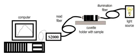
A typical configuration for an absorbance experiment.
