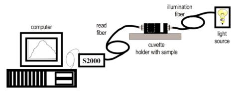
A typical configuration for a transmission experiment.
