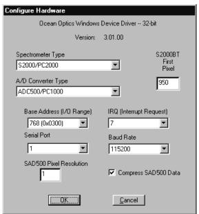
If you do not see the "Configure Hardware" screen, exit the software. Then select **Start** | **Run**, and type C:\windows\ooidrv.ini. Notepad will open. Edit this file for our device driver by finding the "Initialized" entry and making sure this line reads **Initialized=0**. Save the OOIDRV.INI file and exit Notepad. Restart OOIBase32. You should now see the "Configure Hardware" dialog box.
