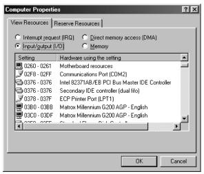
For most computers, the default settings work well. In the picture above left, it appears that the Printer occupies IRQ 07, but for most computers, our A/D converters can share the IRQ 07 setting with a printer and conflicts will not arise. All computers have multiple Base Address (Input/output) settings from which to choose.
