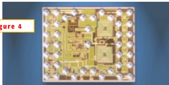
The Silicon-Germanium RF chip used in IBM 's 12-channel GPS module that measures 66 × 40 × 4.5 mm, features rapid time-to-first-fix and runs on a 3.3V supply
