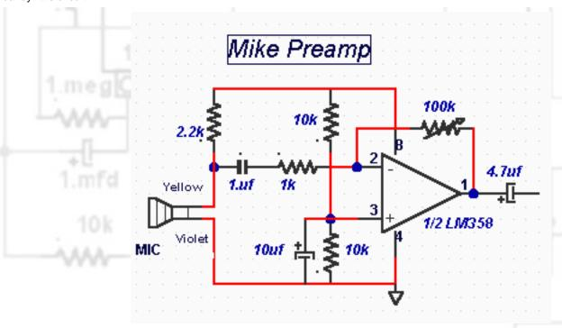
The circuit below is a complete circuit for use as a powerful microphone amplifier with a gain of up to 4000.
